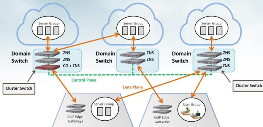
*A large-scale CoIP configuration, with multiple cloud and enterprise domains, along with clustering of network switches (ZNS), managed by a master controller gateway (CG).*
